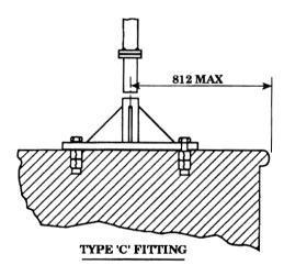
ABOVE FLOOR MOUNTING ON SOLID CONCRETE BASE BASE PLATE ASSY. PT No. A977 FIXED WITH EXPANDING BOLTS
